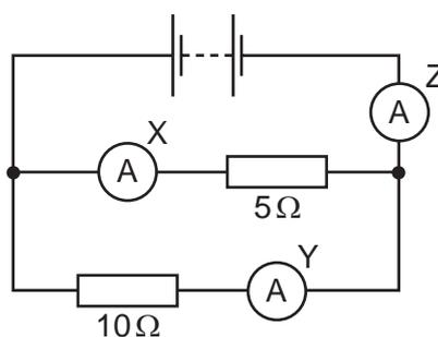
The ammeter readings are 1 A, 2 A and 3 A.
